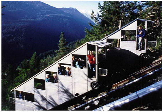
The Châtelard VS historical Funicular (1920) holds the world record for the steepest two-carriage service (87%)
